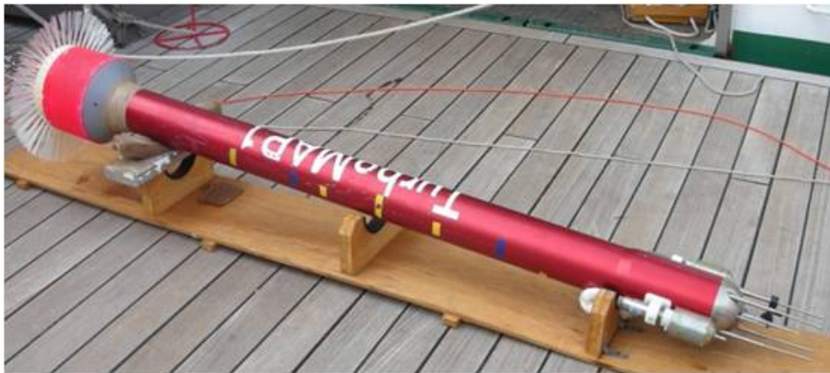
Figure 3.4: TurboMAP - a photograph of the microstructure profiler TurboMAP: Turbulence Ocean Microstructure Acquisition Profiler
