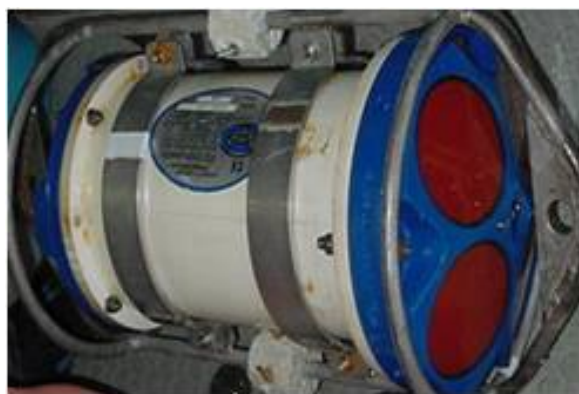
Figure 3.6: ADCP - a photograph of one of the five ADCPs deployed at the mouth of Shiozu Bay
