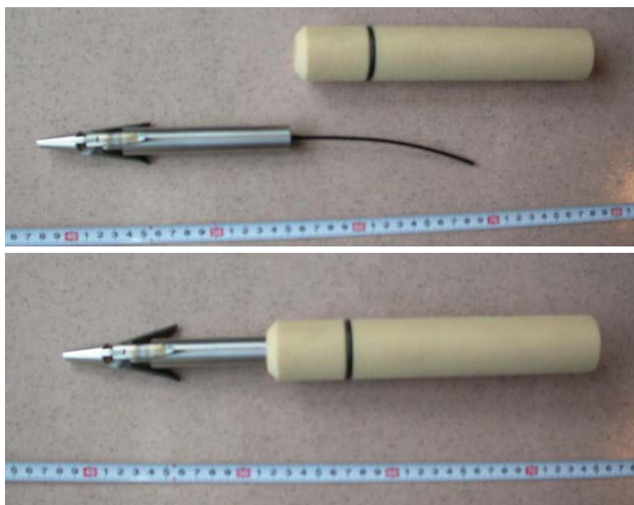
Fig. 4-4. Darts used in the tagging experiment with an air gun in 2004. Upper photograph indicates dummy tag and a retrievable float. Lower photograph indicates tag with the float at firing.
