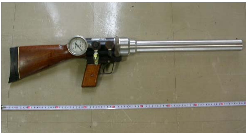
Fig. 4-3. Air gun used for attachment of the satellite tags in 2004 to 2008.
