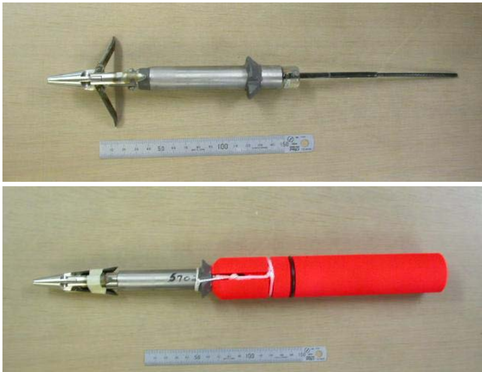
Fig. 4-6. The satellite tag used for Bryde's whales in 2004 to 2008. Upper photograph indicates Argos transmitter with dart and stopper. Lower photograph indicates the tag with a retrievable float.
