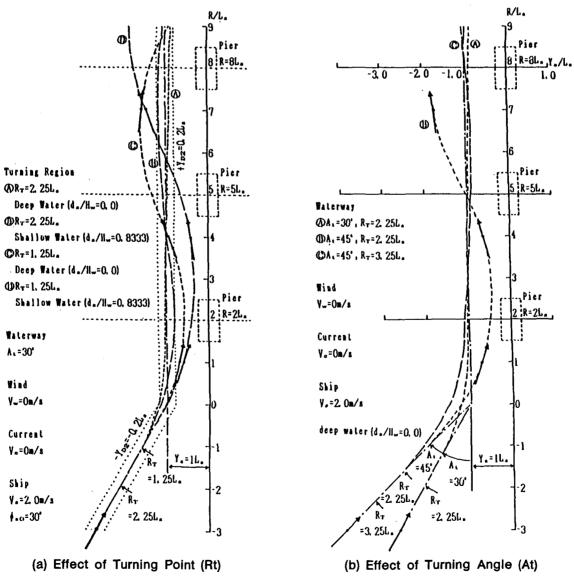
Fig.12 Ship's Trajectories affected by Waterway
