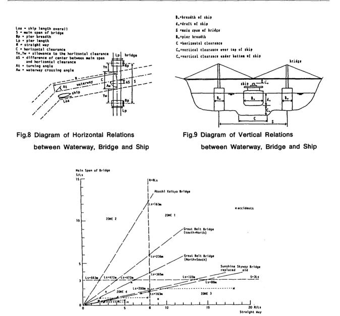
Fig.10 Main Span of Bridge and Straight Way related to Ship's Size
