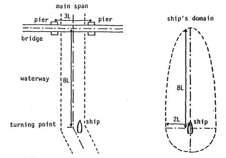
Fig.11 Waterway Passing through Bridge and Ship's Domain
