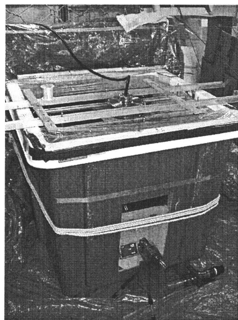
Fig. 1. Target strength measurement system using the split-beam method and a small tank.
