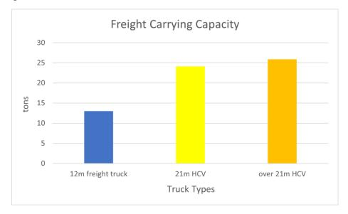
Fig. 2.11 Increase in freight carrying capacity (source: MLIT, 2019)
