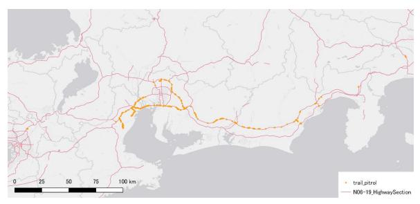
Fig. 4.26 High trailer rolling/pitching points
