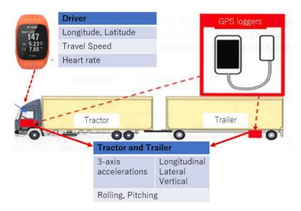
Fig. 3.2 Data logger on an HCV (source: Watanabe and Hyodo, 2020)
