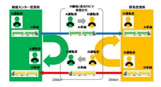
Fig. 2.12 Relay transportation (source: MLIT, 2019)
