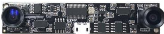
Fig. 2-6: ELP-1MP2CAM001-HOV90 dual-lens camera module
