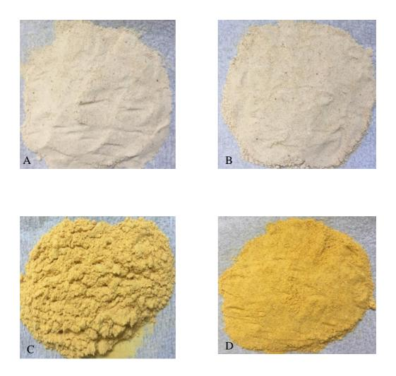
Figure 2. Final product after extrusion, extrudates A (SBM, 100°C), B (SBM, 150°C), C (CGM, 100°C), D (CGM, 150°C)
