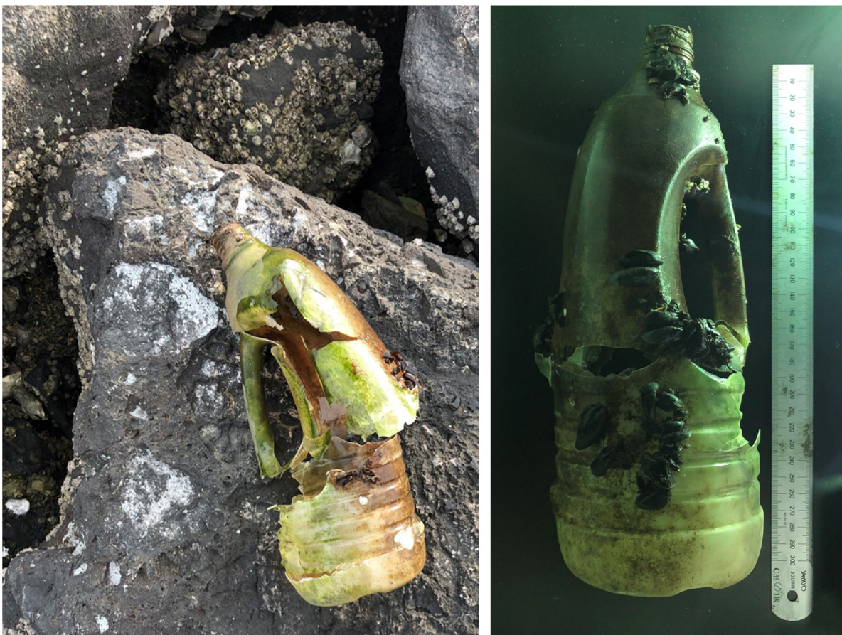
Figure 3.1.1. Biofouling organisms such as algae, mussels and barnacles that have grown on an ethylene-butyl acrylate plastic bottle. The left side of the Figure shows the situation in the field where the bottle is located, and on the right side, it is shown together with the scale in the laboratory. In addition, it showed one side of the bottle in two photographs and conveyed the biofouling organisms on it.
