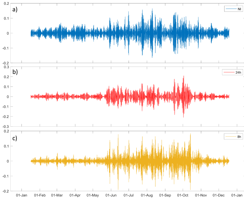
Figure 4.7. Inverse CWT derived current velocity, in \text{m s}^{-1} , for (a) the inertial band, (b) the diurnal band, and (c) the 8h period band at 82 m deep.
