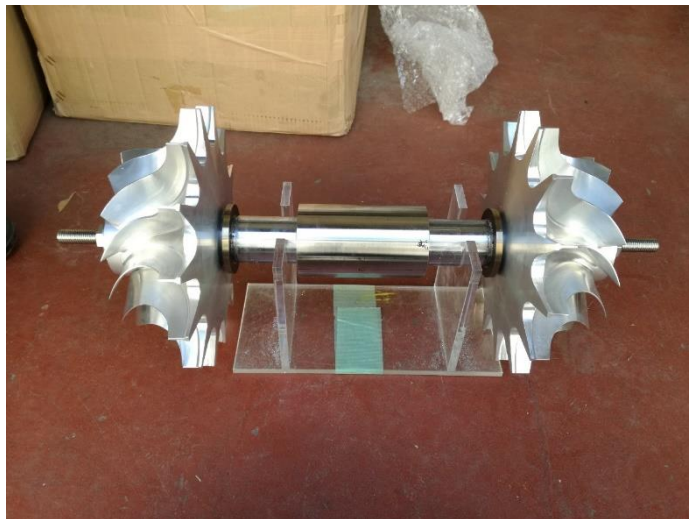
Fig. 18 Radial twin turbine, turbine shaft and permanent magnet
