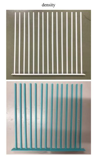
Fig.2.2.13 Flexible (top) and rigid (bottom) vegetation models
