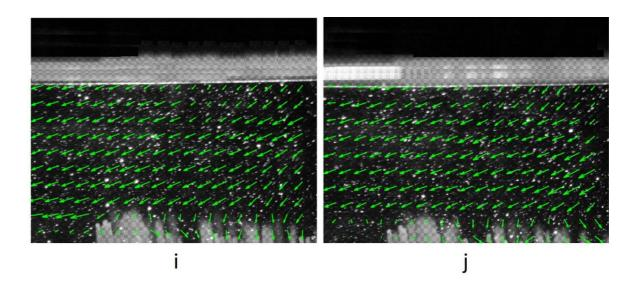
Fig.3.4.3 The result of instantaneous velocity fields with flexible vegetation model
