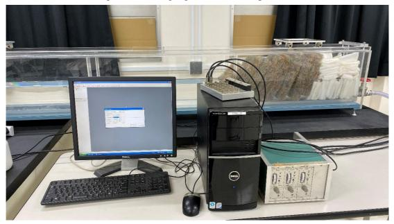
Fig.2.2.6 Data capturing system for the wave gauges
