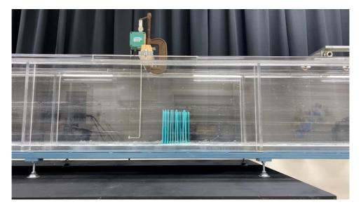
Fig.2.3.15 Snapshot for rigid vegetation model
