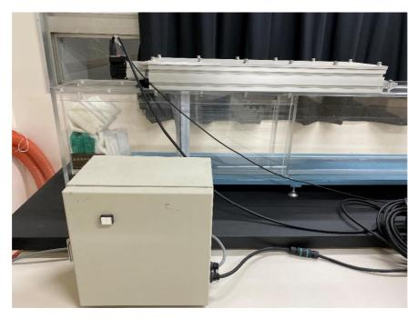
Fig.2.2.3 Wave generation system of the flume
