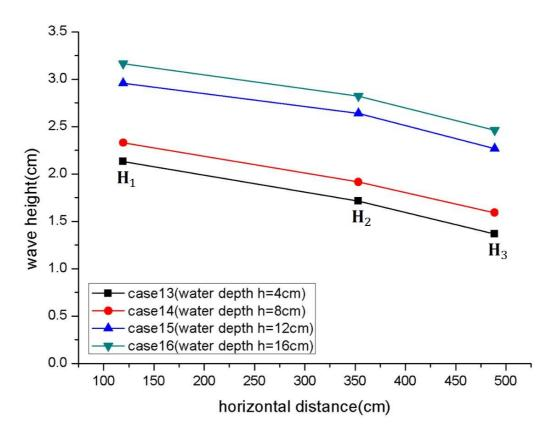
Fig.2.3.16 The result of wave height along horizontal distance with flexible vegetation
