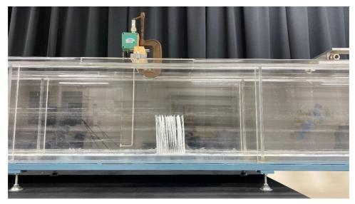
Fig.2.3.14 Snapshot for flexible vegetation model
