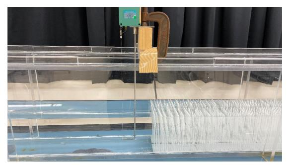
Fig.2.2.5 Wave gauge used in the experiment
