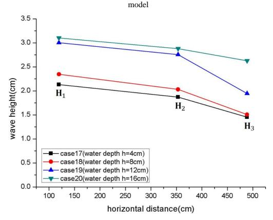
Fig.2.3.17 The result of wave height along horizontal distance with rigid vegetation model
