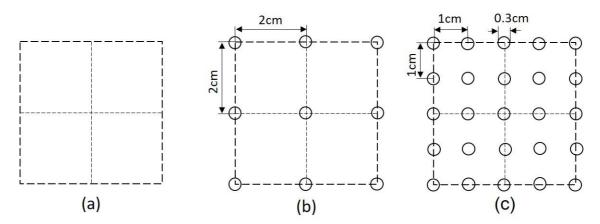
Fig.2.2.12 Vegetation model arrangements. (a)No vegetation, (b)Low density, (c)High
