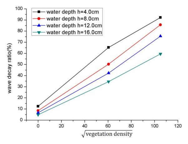
Fig.2.3.13 The result of wave decay ratio along the square root of vegetation density
