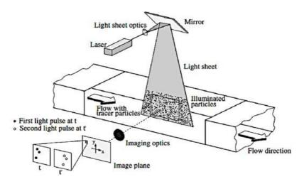
Fig.3.2.1 Sketch of a typical laboratory PIV system (Raffel et al, 2007)
