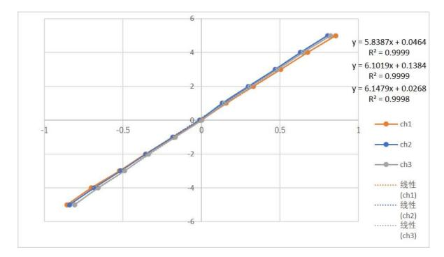
Fig.2.2.7 Calibration data of the wave gauges
