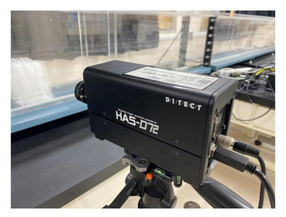
Fig.3.3.5 High-speed CCD camera
