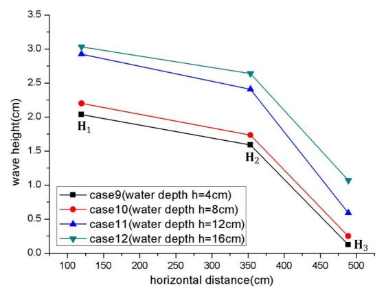
Fig.2.3.11 The result of wave height along horizontal distance with high vegetation density
