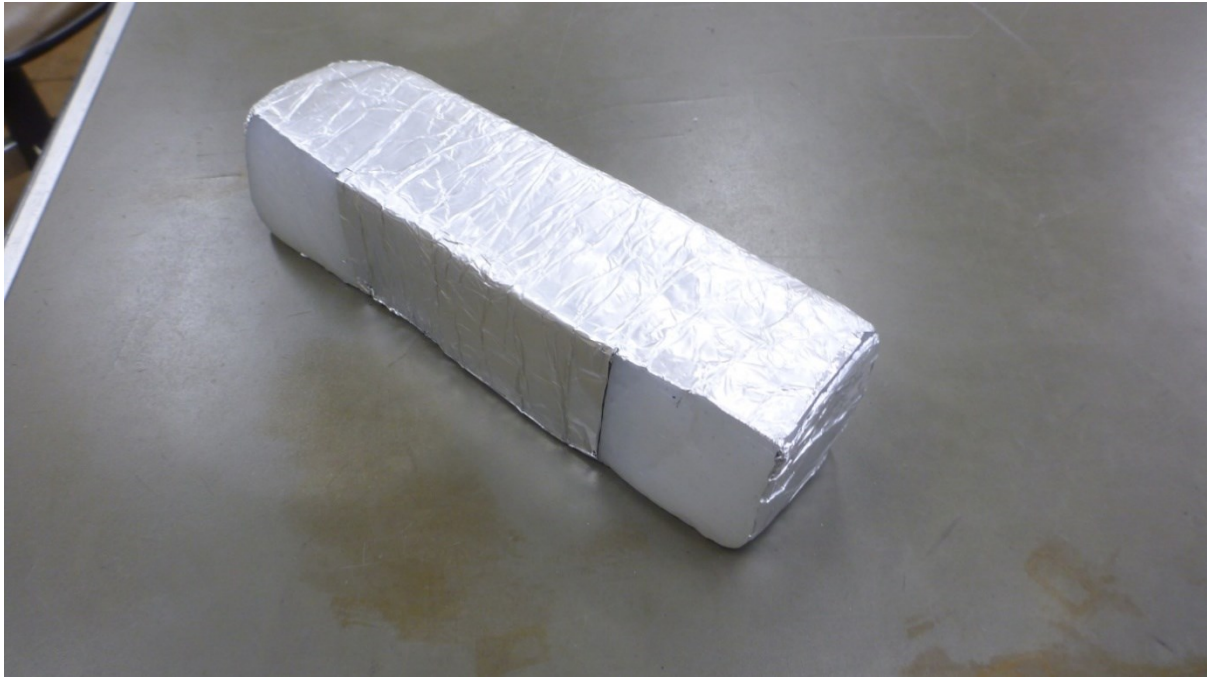
Fig. 5-4 Propagation Channel Wrapped by Aluminum Foil (Length 200[mm])
