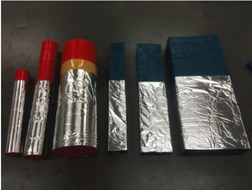
Fig. 5-9 Propagation Channel Wrapped by Aluminum Foil for Communication Capacity
