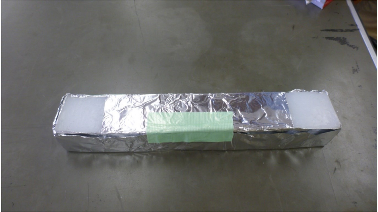
Fig. 5-3 Propagation Channel Wrapped by Aluminum Foil (Length 300[mm])
