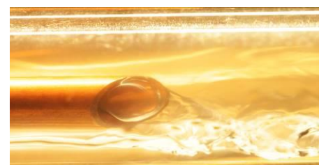
Fig.4.3 Typical flow pattern of R32 for smooth tube(SM)
