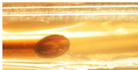
(b) Wavy flow G = 100 \text{ kg m}^{-2} \text{ s}^{-1} , 1-x = 0.69
