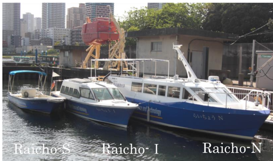
Fig. B.1 Quick-charging compatible battery power electric boats "Raicho I", "Raicho S" and "Raicho N"
