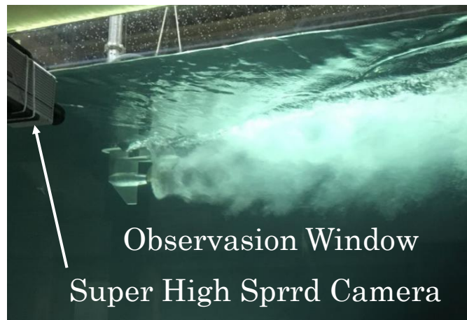
Fig. 3.5 Observation window of horizontal circulation water channel
