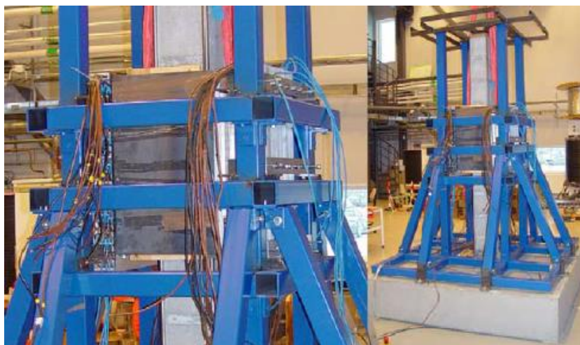
Fig. 1-10 A 10 kW laboratory four-sided, three-phase synchronous linear generator [45].
