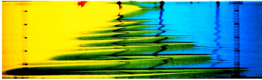
Fig. B.2 Horizontal interleaving experimented by Ruddick and Turner (1999) Blue water is cold/fresh, Yellow is warm/salty.
