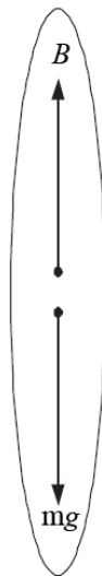
Figure 2.6: Vertical profiler in static equilibrium - A vertical profiler in static equilibrium with its surrounding fluid. Its weight is represented by mg and its buoyancy is represented by B .
