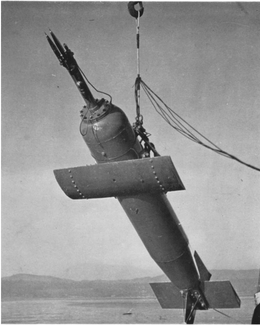
Figure 1.5: The first towed vehicle to measure oceanic turbulence - A converted minesweeping paravane. Photo extracted from Grant et al. (1962).
