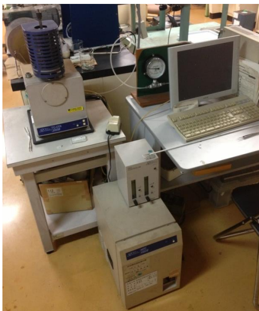
Figure 2-2 Photograph of our TG-DTA system (MAC Science, WS002).
