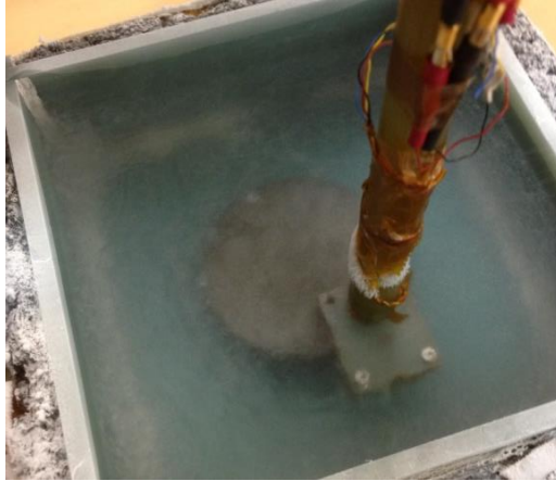
Figure 6-1 Schematic view of trapped field measurement in our laboratory.
