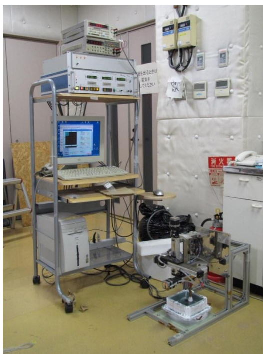
Figure 2-4 Photograph of the automatic Hall probe measurement system.
