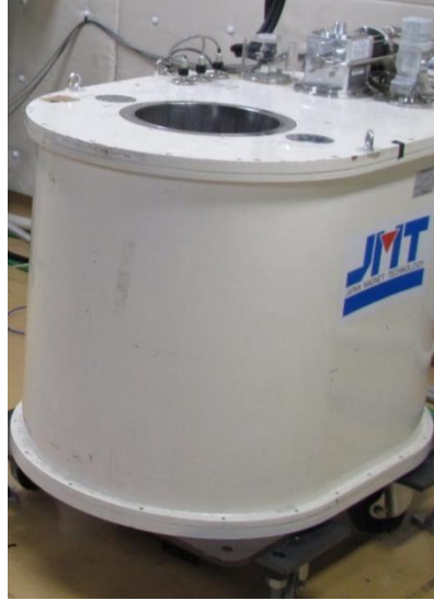
Figure 2-5 5 T superconducting magnet.
