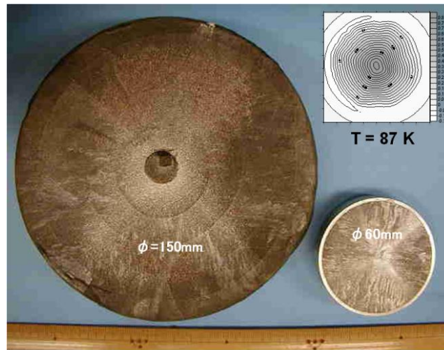
Figure 1-10 The fabricated single domain bulks by employing TSMG technique. The large bulk has a diameter of 150mm. The small one has a diameter of 60mm. Inset illustrate the flux distribution in the large bulk. (Hidekazu Teshima, Nippon Steel, Japan)
