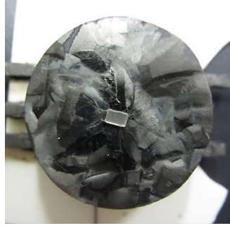
Figure 2-18 Image of the Mg-doped Nd-123 textured by using MgO seed.
