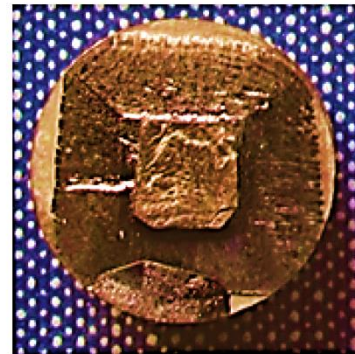
Figure 2-15 A single domain obtained by using the optimal temperature profile in fig. 2-14.
