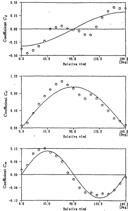
Fig.2 Wind Effects,  $C_x, C_y$  and  $C_N$
