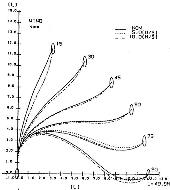
Fig.16 Paths of the Minimum-Time Inward Stopping with Wind Blowing Off
