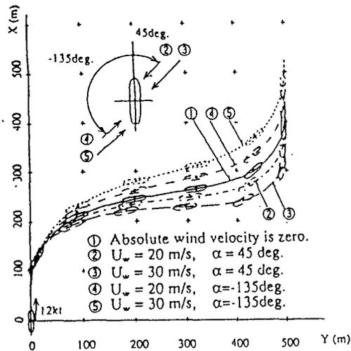
Fig.3 The Calculated Paths of Minimum Deviations with Winds
