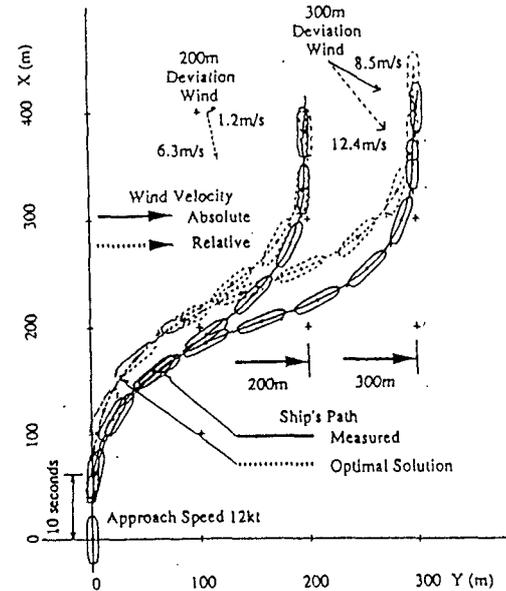
Fig.5 The Paths of the Actual Automatic Deviation Tests
