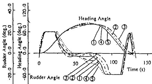
Fig.4 The Calculated Time Histories of Rudder Angles and Heading Angles
