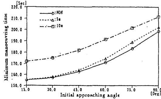
Fig.8 The Minimum Inward Stopping Times with the Wind Blowing On
