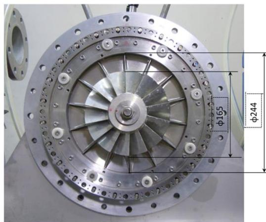
Fig. 10 Installed Radial Turbine
