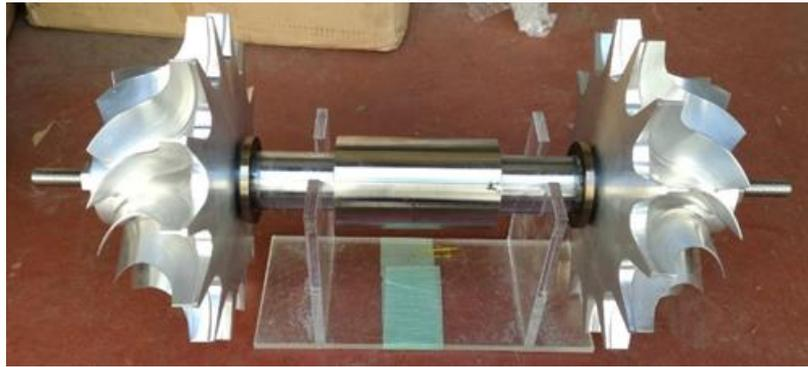
Fig. 9 Radial Twin Turbine, Turbine Shaft and Permanent Magnet
