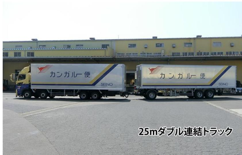
Fig. 1.6 A 25m HCV in Japan (source: MLIT, 2019)
