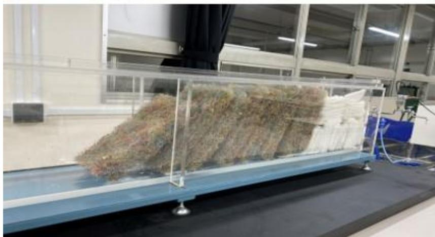
Fig.2.2.4 Absorbing materials on both ends of the wave flume
