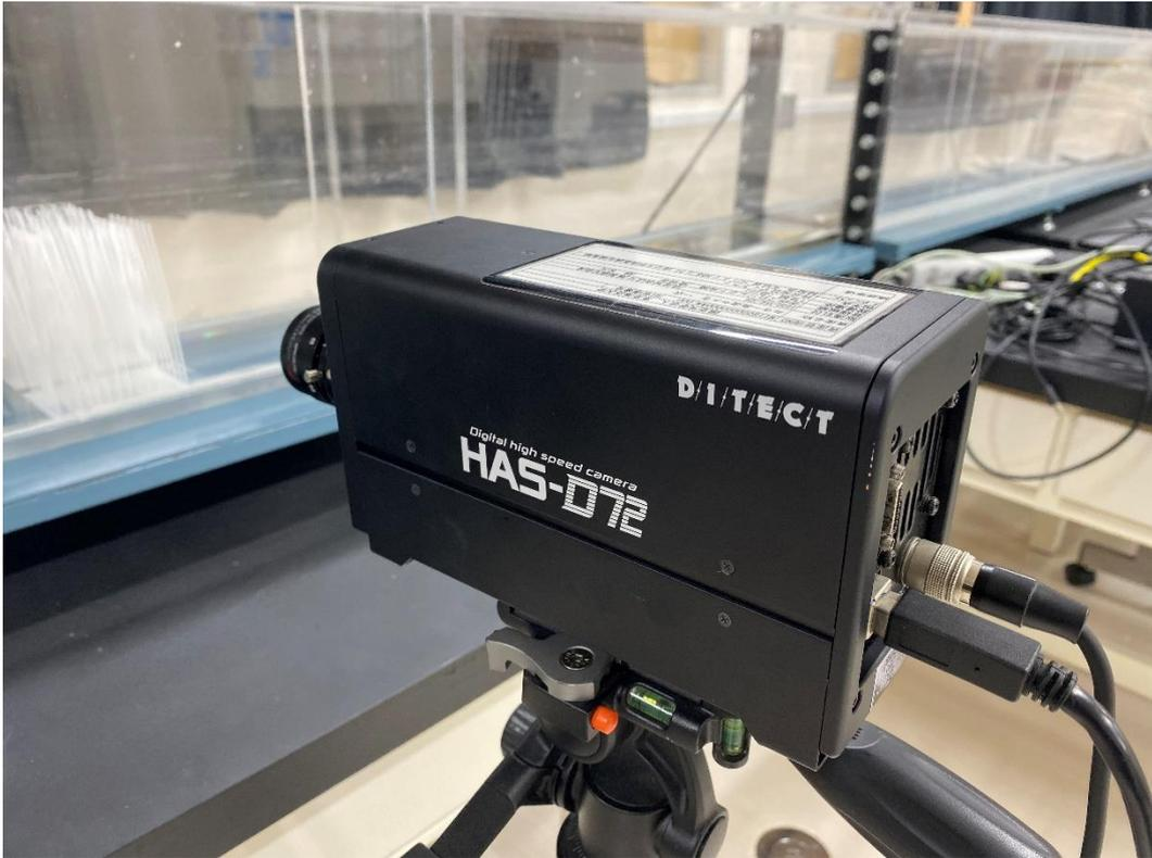
Fig.3.3.5 High-speed CCD camera
