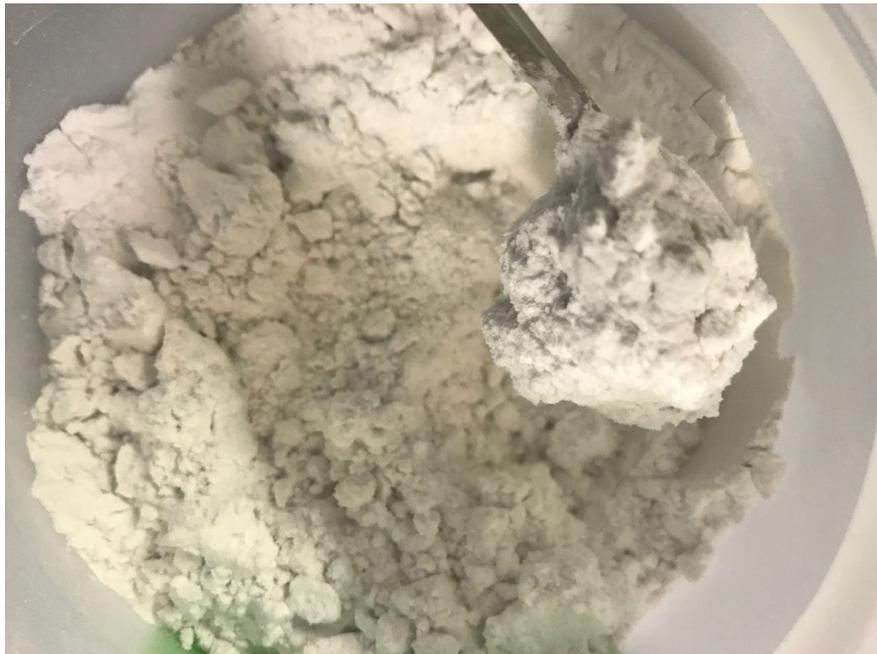
Figure 4.6 The photo of tracer particles(HGS, diameter=10 $\mu$ m)
