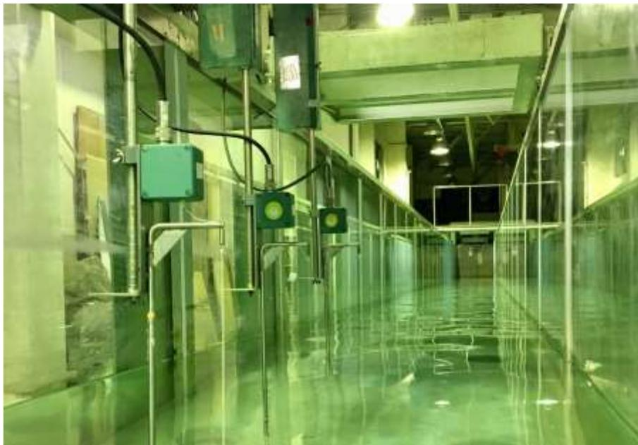
Figure 3-9 CHT6-50E 2-line Capacitance Type Wave Gauges.
