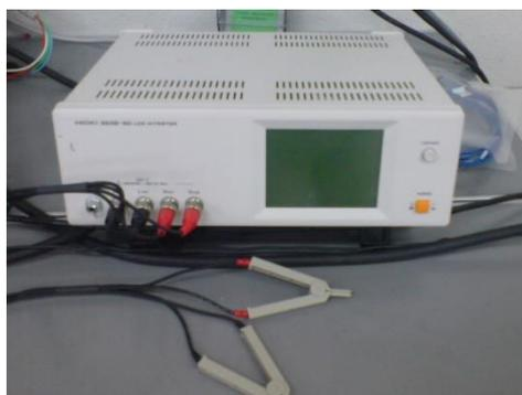
**Fig. 2-2** LCR meter (HiTESTER3532-50, HIOKI Co. Ltd., Japan)
