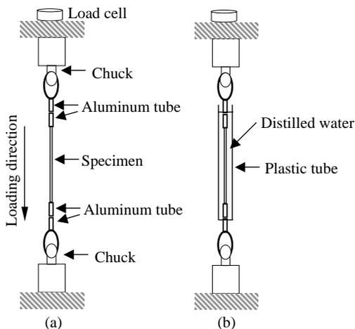
**Figure 1.** Scheme of tensile and fatigue experiments. A specimen set on the chucks. (a) dry condition. (b) wet condition.
