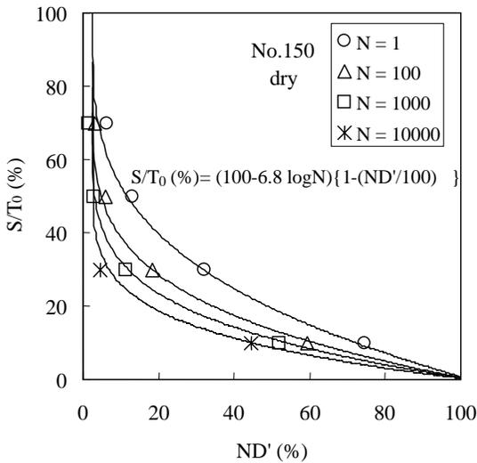
Figure 12. Fatigue life curves calculated from equation (5).
