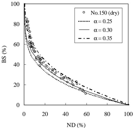
**Figure 6.** Calculation curves for some different  $\alpha$  values by the equation (1) with observed data of No.150 nylon monofilament.
