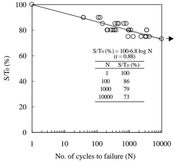
**Figure 9.** Relationship between imposed load ( $S/T_0$ ) and number of cycles to failure of un-notched filament ( $S/T_0$  (%) =  $a - b \log N$ ;  $a = 100$ ,  $b = 6.8$ ).  $r$ : coefficient of correlation. An arrow indicated the specimen that did not break within  $10^4$  cycles of the testing.
