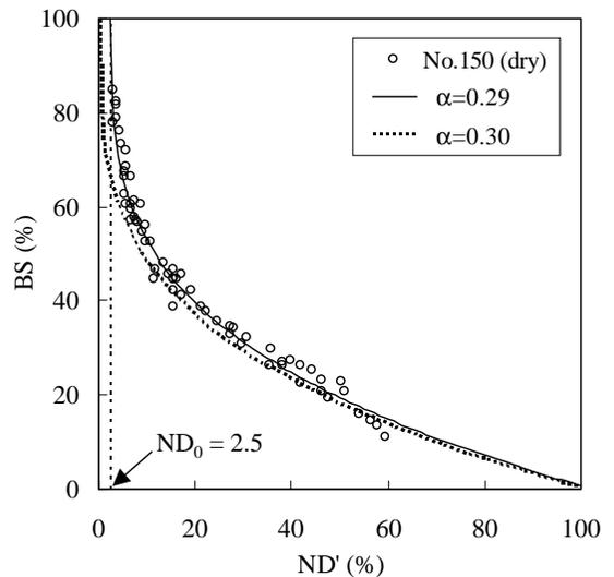
**Figure 7.** Calculation curves for relationship between breaking strength and notch depth with observed data of No.150 nylon monofilament.  $BS = 100 \{1 - (ND'/100)^\alpha\}$ . Where  $ND' = ND + ND_0$ .
