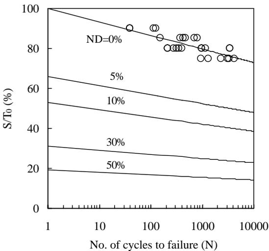
Figure 12. Relationship between imposed load and number of cycles to failure of notched nylon monofilament.  $S/T_0$  (%) =  $(100 - 6.8 \log N) \{1 - (ND/100)^\alpha\}$ ,  $\alpha = 0.29$ . Solid lines at various notch depth were calculated at constant  $\alpha = 0.29$ .
