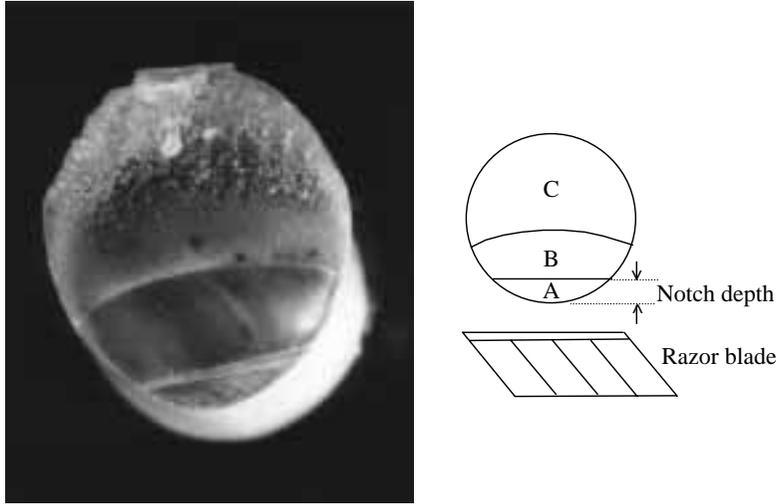
**Figure 3.** Failure surface of a notched sample (A: Razor notch, B: Area of ductile fracture, C: Area of brittle fracture).
