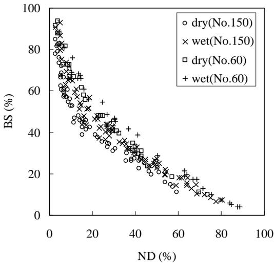
**Figure 5.** Relationship between retained breaking strength (%) and notch depth (%) of dry and wet nylon monofilament (No.150 and No.60).
