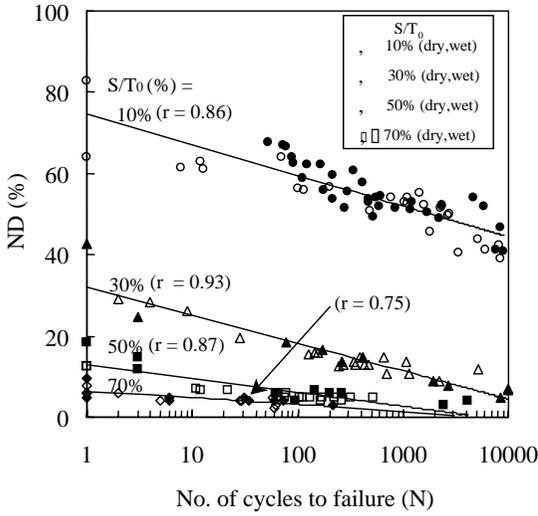
**Figure 10.** Relationship between notch depth (%) and number of cycles to failure for dry and wet nylon monofilament (No.150).
