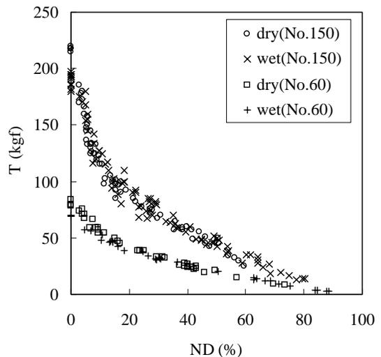
**Figure 4.** Relationship between tensile strength (kgf) and notch depth (%) of dry and wet nylon monofilament (No.150 and No.60).
