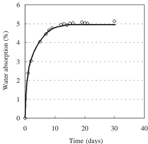
**Figure 2.** Changes in water absorption of nylon monofilament. Water absorption (%) =  $((W_t - W_0)/W_0) \times 100$ . Where  $W_0$  is the initial weight (g) of tested sample and  $W_t$  is weight (g) after immersion,  $t$  (days).
