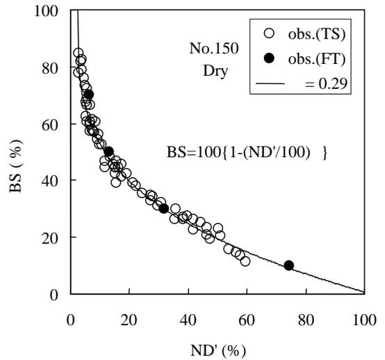
**Figure 11.** Fatigue life curve for fatigue data. : tensile observed data referred to Fig. 8(a), : the value of ND(%) and  $S/T_0$  (%) were calculated from equation (4), ND values at constant imposed load (10, 30, 50 and 70%) were estimated by extrapolating at  $N = 1$ .
