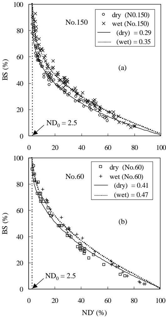
**Figure 8.** Calculation curves for relationship between breaking strength (%) and notch depth (%) of four specimens (dry and wet for both No.150 and No.60 nylon monofilament).
